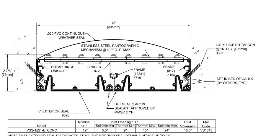
NOTE THAT EXTERIOR SEAL DISENGAGES AT 19". THE INTERIOR SEAL REMAINS INTACT UP TO 24".
